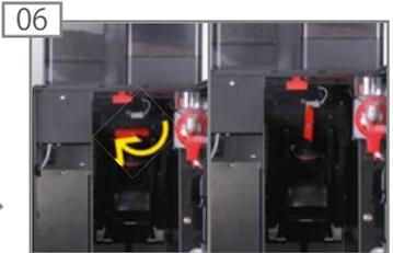
06 Lock the brewing module in clockwise direction.
